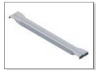
The pallet support is used to support pallets of poor quality or when pallets are placed with the I200mm side facing the aisle. A pair of galvanised cold-rolled pallet supports can take a load of up to I200kg.
