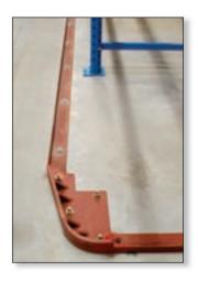
This type of racking is operated with "very narrow aisle" trucks. They are guided through the aisle, allowing faster and easier operation. Inductive guidance often replaces the rail guidance.
