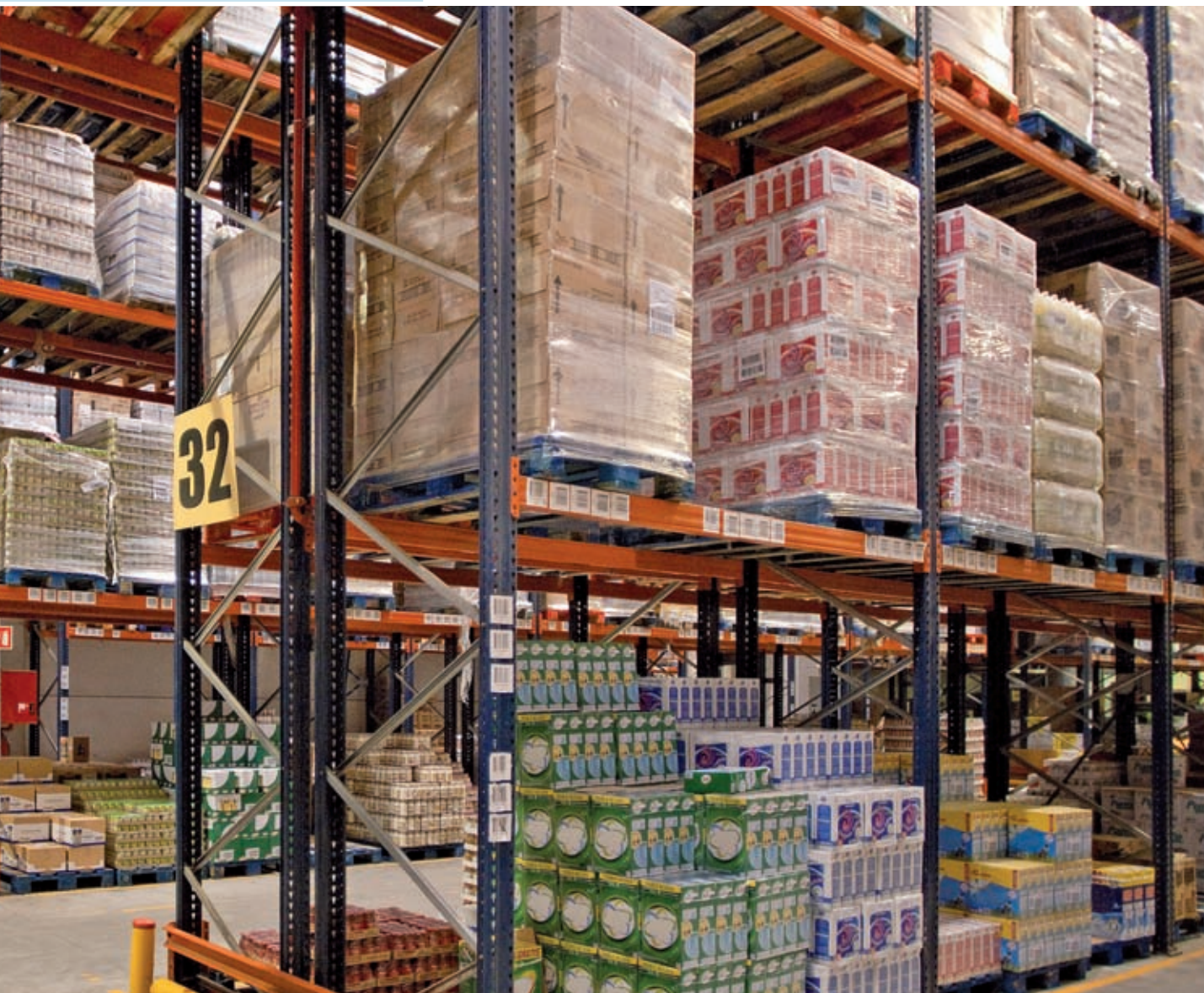
Conventional pallet racking warehouse. Pallet handled by side measuring 800 mm.
